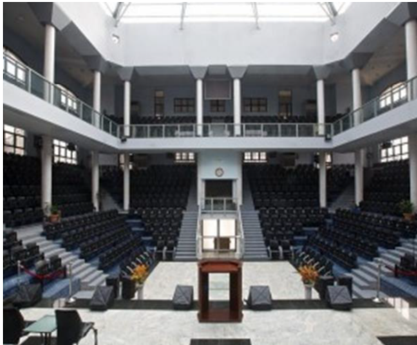
Plates 3: Showing a large skylight covered central atrium allowing light influx into the Auditorium.
